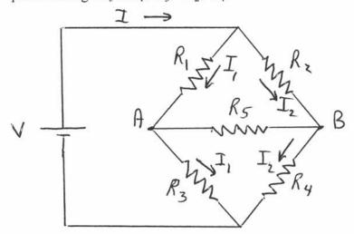
No current through  $R_5 \Rightarrow V_{AB} = 0$ . Lack across  $R_1 = valtage$  across  $R_2$  $I_1R_2 = I_2R_2$  (1)
