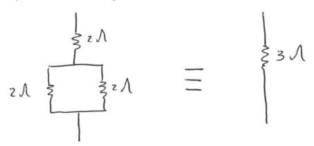
b) Show that the total power dissipated in the above circuit is the same as when a single 3 ohm resistor is available.
