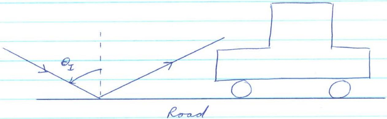
Sunlight heats the road producing a layer of warm air near the surface. At the boundary between warm + cool air, light is reflected and transmitted. P polarized light incident at an angle  $\theta_I \approx \theta_{\text{Brewster}}$  is not reflected.  $\therefore$  the reflected
