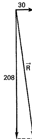
Fig. 3.12. The resultant velocity is found by means of the parallelogram of velocities.
