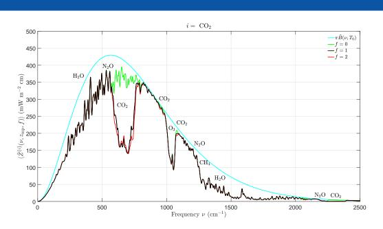
Figure 5: The spectral forcing at current levels of carbon dioxide,  $CO_2$ , (the black curve with f = 1), or if concentrations of carbon dioxide are doubled (the red curve with f = 2), or if all carbon dioxide is removed (the green curve with f = 0). See the caption of Fig. 4.
