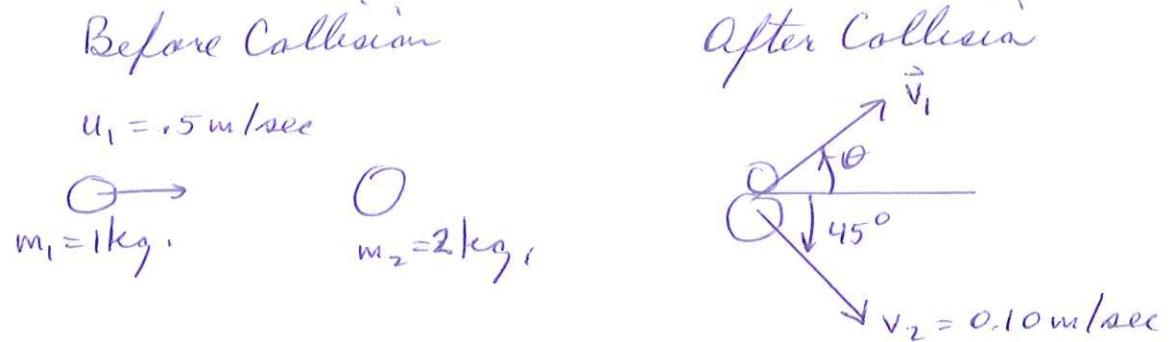
Cons. of  $p_x:$   $m_1 v_1 = m_1 v_1 \cos \theta + m_2 v_2 \cos 45^\circ$
