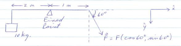
How large must F be to balance the 10kg. mass?
