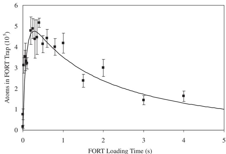
**Fig. 7.** Time evolution of atoms in FORT after QUIC trap was turned off.
