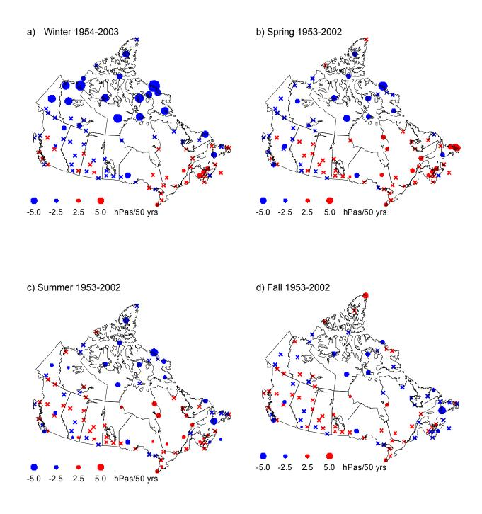
Fig. 2: Trend in Surface Pressure During a) Winter; b) Spring; c) Summer; d) Fall. Blue (red) dots represent decreasing (increasing) surface pressure statistically significant at the 5% level. Crosses represent insignificant trends.
