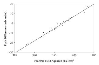
**Fig. 4.** Stark shift data of  $3D_{5/2} |m_J| = 3/2$  state. The laser was scanned across the resonance and the electric field was varied to determine the field strength such that the  $3D_{5/2}$  peak excited in the field free region by the laser frequency sideband shifted by 995.000 MHz was simultaneously excited as the  $3D_{5/2} |m_J| = 3/2$  peak in the field region. The electric field needed to overlap the two peaks was found using a linear fit to be  $19.611 \pm 0.008 \text{ kV/cm}$ .
