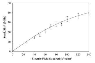
**Fig. 5.** Sample stark shift data of  $3D_{3/2}|m_J| = 3/2$  state. The data was fitted to a curve  $y = A_0 \mathcal{E}^2 + A_1 \mathcal{E}^4$  as described in the text.
