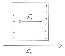
Inside the conductor,  $\vec{E}_o$  drives positive charge to the right surface and negative charge to the left surface. These so called induced charges produce a field  $\vec{E}_1$  opposing  $\vec{E}_o$ . Charges continue to move until  $\vec{E}_1$  exactly cancels  $\vec{E}_o$ . The time for this movement of charge to occur is extremely short. Hence, we conclude that inside a conductor the electric field is zero.
