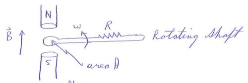
The magnetic going through the loop is given by  $\Phi(t) = B A \cos \omega t$ . The voltage across the resistor is then found to be  $V = -d\Phi / dt$ .
