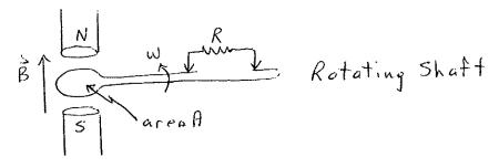
The magnetic flux going through the loop is given by  $\Phi(t) = B A \cos \omega t$ . The voltage across the resistor is then found to be  $V = -d\Phi/dt$ .
