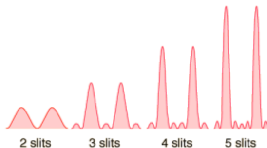
Figure 10.3: Narrowing of Interference with more slits.
