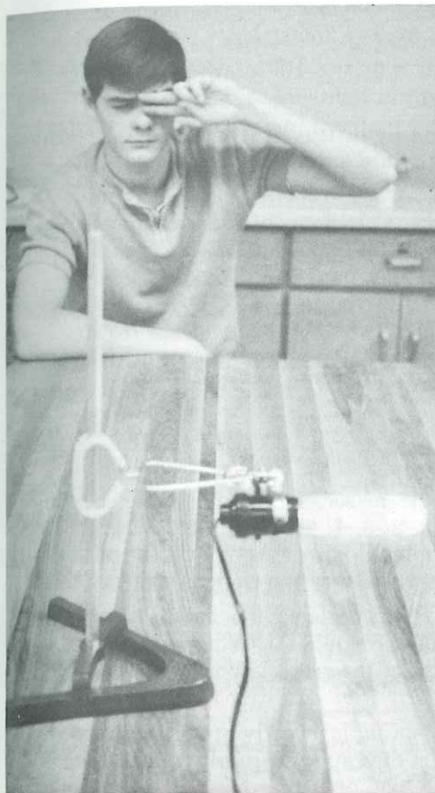
Fig. 1.14. Diffraction of light becomes evident when a narrow source of light is viewed through a narrow opening between two fingers.
