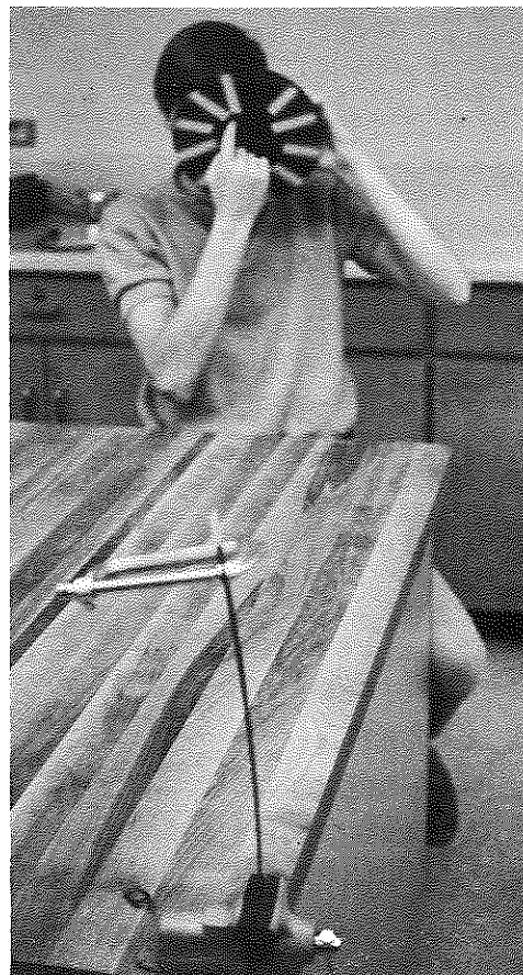
Fig. 4.4. A disc stroboscope in use.
