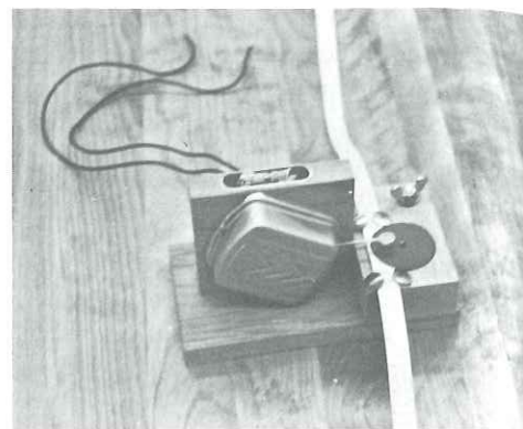
Fig. 4.6. The clapper of the timer strikes the carbon paper on top of the white paper tape. As a result, dots are recorded on the tape as it is pulled through the timer.
