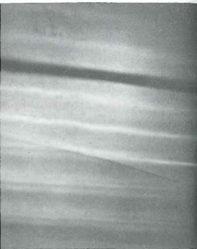
Fig. 4.26. Low frequency straight waves are refracted as they pass from deep water (bottom) to shallow water (top). The black marker is parallel to the refracted waves.
