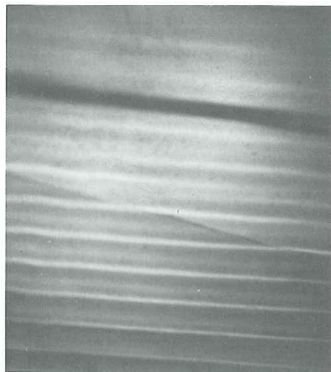
Fig. 4.27. For waves of higher frequency, the amount of refraction is less. The refracted waves are not parallel to the black marker in this case.
